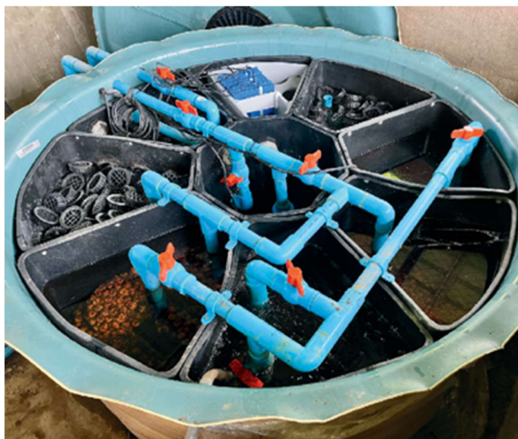
FIGURE 11: Top view from interior of Aquonic module without lid. Source: Documentation by UPM GmbH team during a visit to SCG, 2022.
